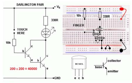
This uses two transistors so the current multiplying effect is much greater. So great in fact that just touching the base connection without completing the circuit is enough to light the LED. Your body is acting as an antenna and picking up all the electrical noise in the room. This is sufficient to light the LED.
